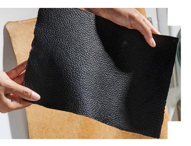
A sustainable leather-like material called Mylo<sup>™</sup>, engineered from mycelium, a fungus that grows naturally Photo courtesy of Bolt Threads
